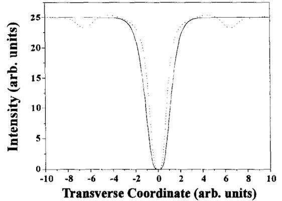
Fig. 3. Radial cross-sections of the input twofold-charged dark beam (solid curve) at high intensity background ( $I = 2.15I_1$ ) and the formed OVS with emitted solitary grey ring (dotted curve) at  $z = 20L_{NL}$ .
