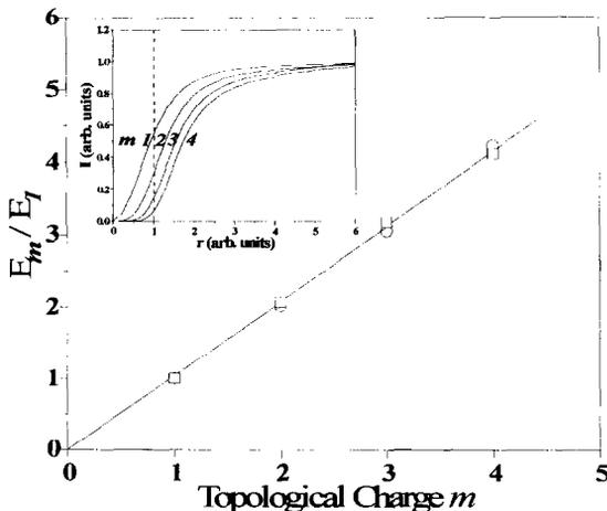
Fig. 2. Normalised soliton constant versus topological charge  $m$  at  $a_m = 1$  (open circles) and  $a_m = 1.5$  (open squares). The solid line presents a linear fit, corresponding to Eq. (8). Insert: Comparison plot of the intensity profiles of multiple-charged OVSs.
