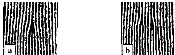
FIG. 7. Interference patterns (converted to black and white) corresponding to an OVS with a TC |m|=2 (a) and to two singly charged OVSs ( z=7 cm, P=60 mW).
