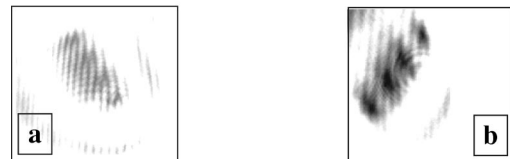
FIG. 11. Gray-scale images of a decayed four-times-charged OVS. The images in (a) and (b) are recorded at P=80 mW and z=6.5 and 7.5 cm, respectively.
