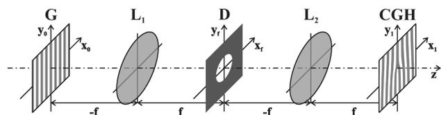
Fig. 1. Illustration of the  $4f$  setup that is analyzed theoretically. G, diffraction grating; CGH, computer-generated hologram with an encoded phase singularity; L<sub>1</sub>, L<sub>2</sub>, lenses of equal focal length  $f$ ; D, iris diaphragm. The input, Fourier, and output planes are denoted by indices 0,  $f$ , and 1, respectively.
