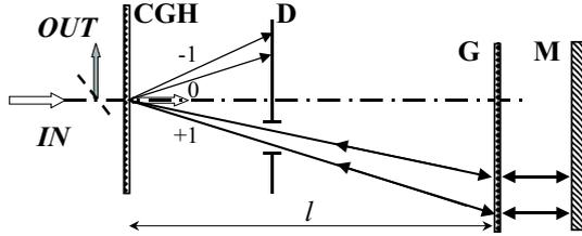
Figure 4. Illustration of the double-pass grating compressor used in [25].  $G$ , diffraction grating;  $CGH$ , computer-generated hologram;  $l$ , compressor length;  $M$  mirror reflecting the beam for the second pass. The CGH is assumed to reproduce the encoded phase singularity at the entrance or at the exit of the compressor.
