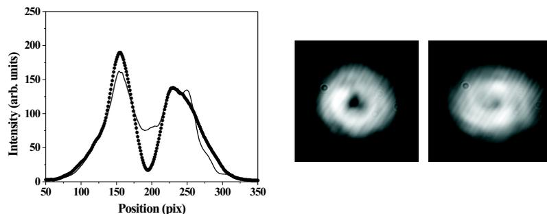
Figure 5. Proof-of-principle experiment and emulation of an optical vortex encoded at the exit of the compressor. Graph: Transverse cross-sections of the uncompensated “idler” (solid) and desired OV (dotted curve). Images: Spectrally integrated experimental frames (compensated OV - left; “idler” OV - right).
