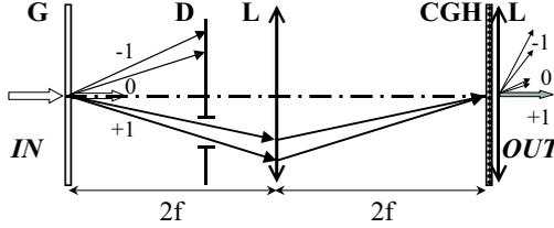
Figure 3. Scheme of the 2f-2f setup used in [24]. The notations are the same as in Fig. 1. Note that the second lens is positioned just behind the CGH (outside the 2f-2f scheme). The CGH is assumed to reproduce the encoded phase singularity at the exit of the pulse stretcher.
