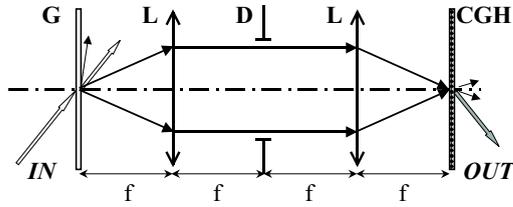
Figure 1. Illustration of the  $4f$  setup analyzed theoretically.  $G$ , diffraction grating;  $CGH$ , computer-generated hologram with an encoded phase singularity;  $L$ , lenses of focal length  $f$ ;  $D$ , iris diaphragm.
