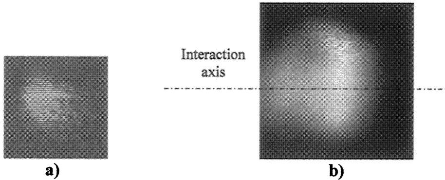
Fig.2. Time-averaged grayscale images of the undistorted (a) and the deflected probe-beam (b).
