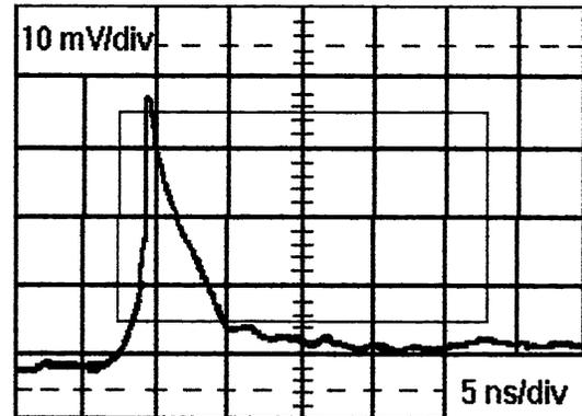
Fig.7a. Optimal pulse shortening (experimental result; detector position - point G on Fig. 3a)
