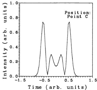
Fig. 6b Initial stage of the formation of a four-pulse sequence. The detector is less offset (Fig. 3b) from the linear probe beam axis than the second peak in the time-averaged pattern of the deflected beam.
