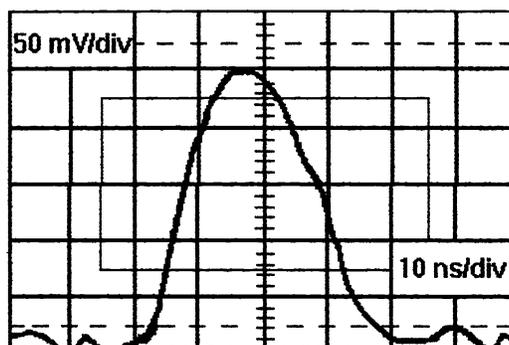
Fig.4. Typical shape of the probe pulses used in the experiment ( $\lambda=532\text{nm}$ )
