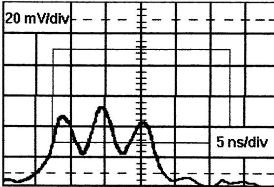
Fig.6a. Sequence of three pulses experimentally obtained with a detector positioned at point C on Fig. 3a.
