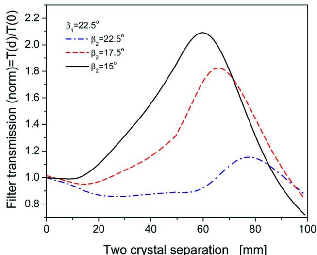
Fig. 2. (Color online) Theoretical dependences of the distance optimization curves calculated for different angles  $\beta_2$  with the model given in Ref. 2 without time integration. The input beam has a radius of  $150\ \mu\text{m}$  (confocal parameter  $\sim 32\ \text{cm}$ ). Normalized input intensity  $S = \gamma_0 |A_0|^2 L = 2$ .
