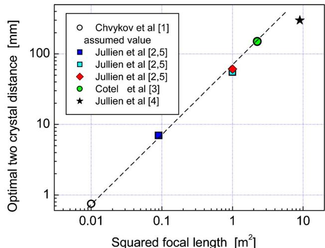
Fig. 1. (Color online) Summary of published optimal distances<sup>1–5</sup> with two-crystal schemes for XPW generation obtained with different focusing of the fundamental beam on the two-crystal setup. The dashed line corresponds to the theoretically predicted slope of 1.
