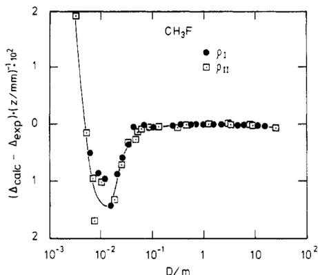
**Figure 3.** Deviation between the calculated and the experimental depolarization ratios for  $\text{CH}_3\text{F}$  plotted as a function of the scaling distance  $D$ , for two near-critical isochores with densities  $\rho_I = 9132.6 \text{ mol}\cdot\text{m}^{-3}$  and  $\rho_{II} = 9190.7 \text{ mol}\cdot\text{m}^{-3}$ .
