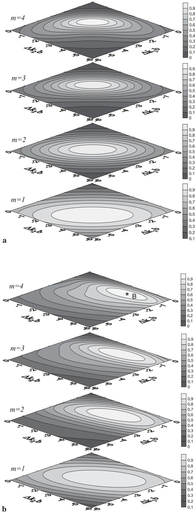
**FIGURE 1** FHG efficiency as a function of both phase matching conditions ( $\Delta k_1 b$ ) and ( $\Delta k_2 b$ ) for two different positions of the focal spot **a**  $l = 0$  and **b**  $l = 0.4$ . Each efficiency distribution is normalized to its own maximum. Normalized input intensity  $S = 0.3$
