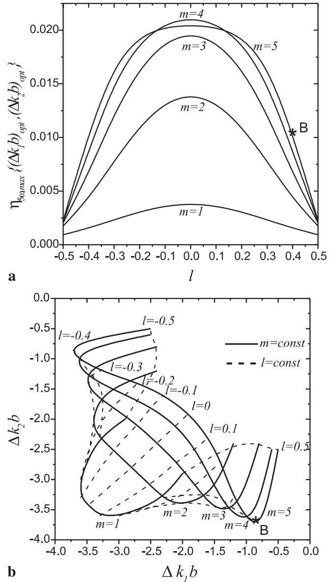
**FIGURE 2** **a** FHG efficiency  $\eta_{5\omega}$  calculated at optimal phase matching conditions as a function of position of focusing  $l$  and **b** optimal phase matching for both steps for several values of level of focusing  $m$  and the position of focusing  $l$ . Normalized input intensity  $S = 0.3$
