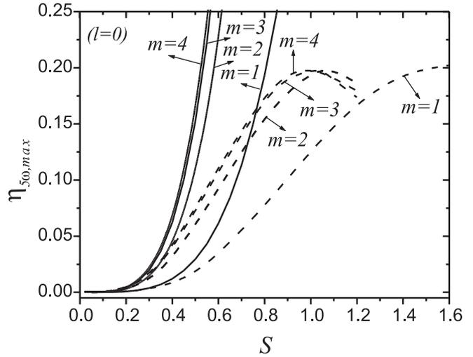
**FIGURE 4** Dependence of FHG efficiency on normalized input intensity. Solid line – calculations with the semi analytical approach given in Sect. 3.2. Dash line – direct numerical integration of system (1) for the case  $\gamma_1 = \gamma_2$
