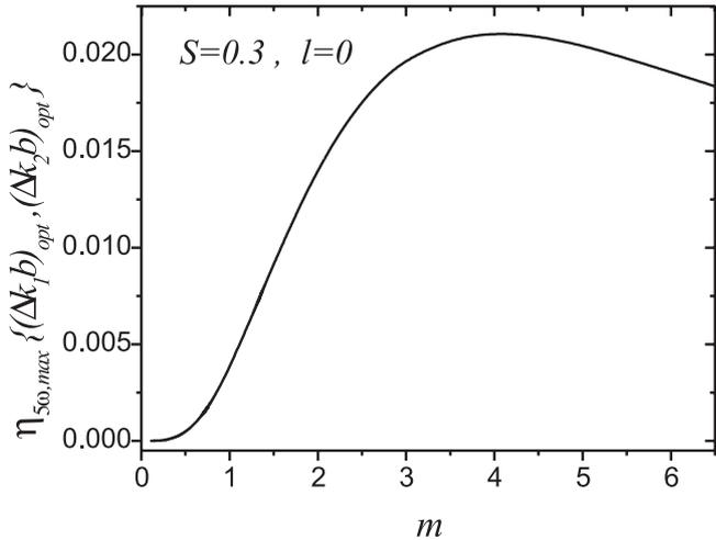
**FIGURE 3** FHG efficiency as a function of the strength of focussing  $m$  for focusing in center of the nonlinear centrosymmetric media
