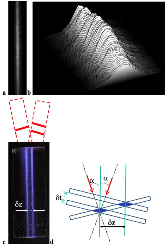
**Fig. 6** (a) Recorded SH trace for two incident fundamental beams at 810 nm and (b) its corresponding transverse profile. (c) Experimental observation of the formation of cross-correlation trace, when one of the fundamental beams carries a sequence of two consecutive pulses. (d) Schematic illustration of this process
