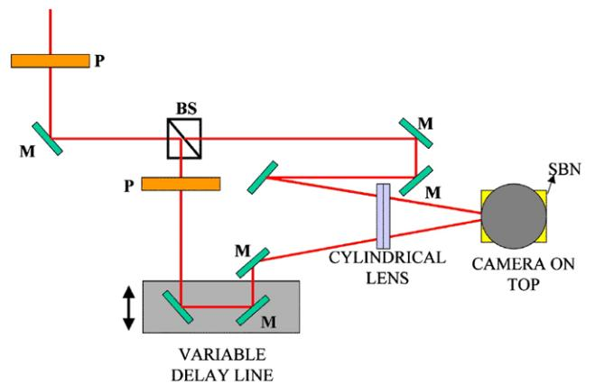
**Fig. 4** Experimental setup. M—mirror, BS—polarizing beam splitter, P—half-wave plates
