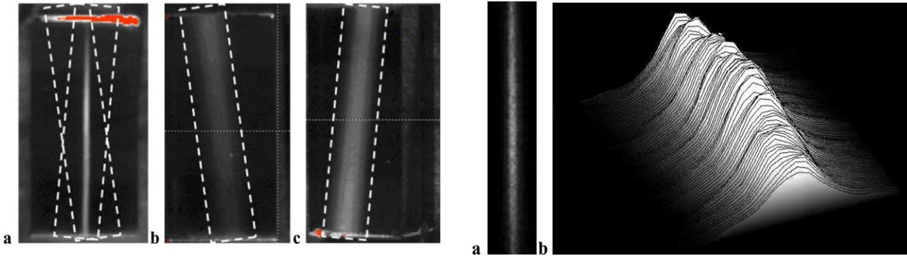
**Fig. 5** Recorded SH traces corresponding to (a) noncollinear planar SHG and (b, c) single beam SHG. To obtain the images (b) and (c), the imaging system is rotated in the  $YZ$ -plane
