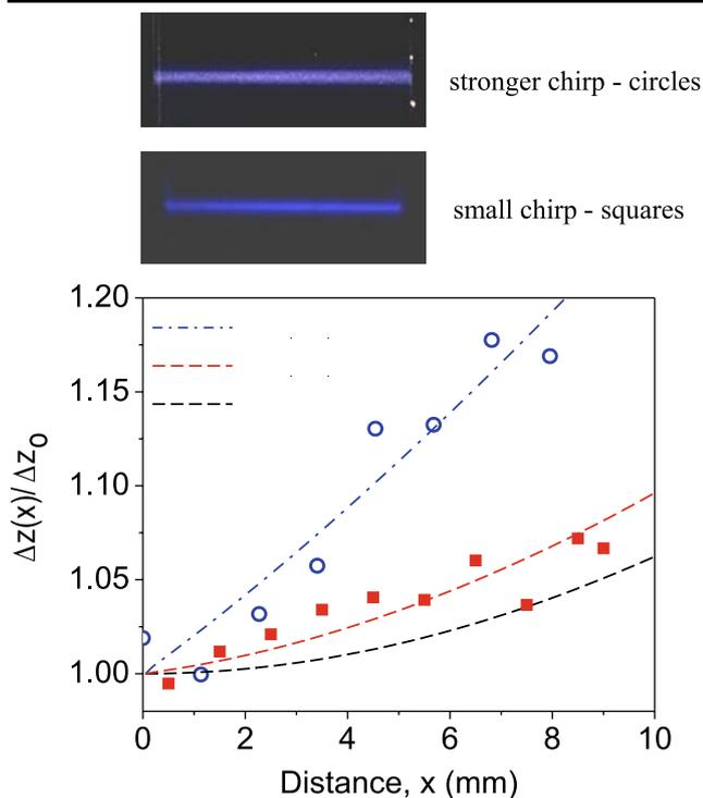
**Fig. 7** Bottom—evaluation of pulse chirp by measuring the transverse width of the SH trace at different locations inside the crystal. Dashed lines represent theoretically calculated evolution of the SH signal for three different values of the incident chirp. Top—two typical autocorrelation traces recorded in the regime of weak and strong chirp
