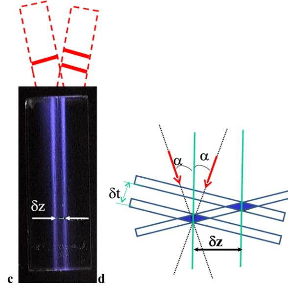
**Fig. 6** (a) Recorded SH trace for two incident fundamental beams at 810 nm and (b) its corresponding transverse profile. (c) Experimental observation of the formation of cross-correlation trace, when one of the fundamental beams carries a sequence of two consecutive pulses. (d) Schematic illustration of this process
