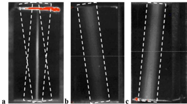
**Fig. 5** Recorded SH traces corresponding to (a) noncollinear planar SHG and (b, c) single beam SHG. To obtain the images (b) and (c), the imaging system is rotated in the  $YZ$ -plane
