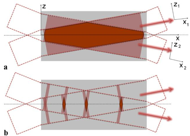
Fig. 2 Beam superposition inside the SBN crystal for the two limiting cases of (a) long pulses and (b) short pulses. For case (b), as beams propagate, the emission region moves along the *X*-axis, giving rise to the recorded trace
